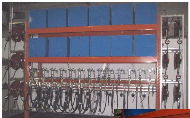
Light armoured equipment manufacturer required a system that would eliminate the clutter and handling of 205 liter drums. System allows for full drums of fluid to be transferred into the tanks on the system. Drums can then be removed or disposed of. A comprehensive pump and hose reel system provides for the efficient and clean transfer and dispensing of the fluids.
